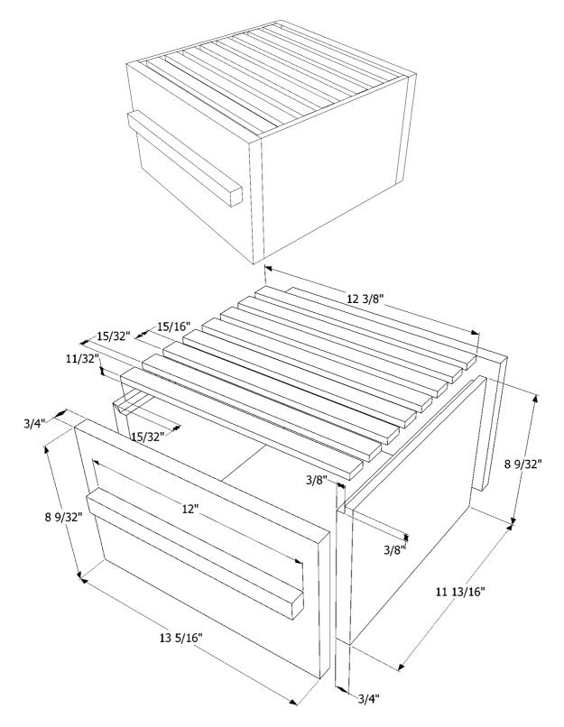
The spacing between all bars and between the end bars and the walls is 15/32". The rebates can be cut with a table saw, a rebating plane or even with a hand saw provided that a guide is affixed to the wood first. Warré specifies a top-bar length of 12 3/8". If it is extended close to 12 9/16", then it better spans the rebates and leaves no cavity for pests to occupy.
