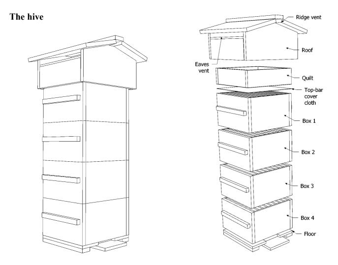
There is no direct passage of air from the top box to the vents under the roof. The quilt is filled with a suitable insulating material of plant origin such as chopped straw, wood shavings, dried leaves etc. As well as a top-bar cover cloth there is a cloth fixed to the bottom of the quilt to retain its contents. A suitable material for these cloths is hessian sacking (burlap).
