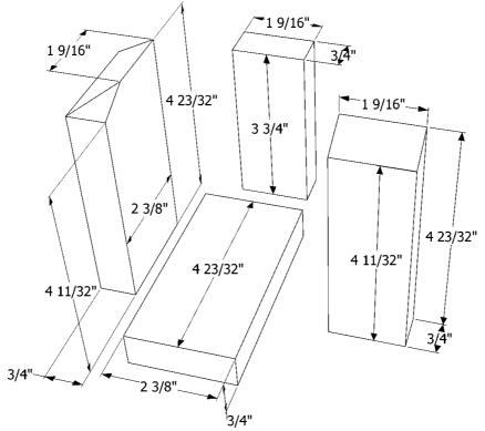
accordingly. The feet may be arranged in a pinwheel (Catherine-wheel) arrangement or constructed as two mirror symmetrical pairs and placed in mirror symmetry accordingly.
