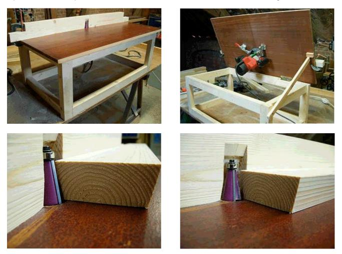
The bit's roller is not actuated because the boards are pressed against the guide instead. The boards are fixed together with false tongue and groove joints. The grooves are made with a 10 mm router bit.
